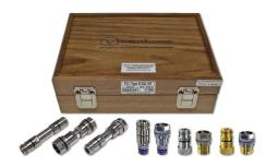
*Warning:* Do not mate 75 ohm type N connectors to 50 ohm type N connectors. Mating a 75 ohm female connector to a 50 ohm type N male connector will destroy the female contact. Mating a 75 ohm male connector to a 50 ohm type N female connector will leave a gap between the male and female contacts which will not provide proper electrical contact for the center conductors.
